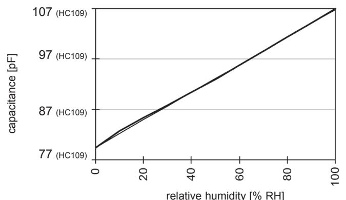
For high accuracy requirements, the sensitivity is determined by the following polynomial:
